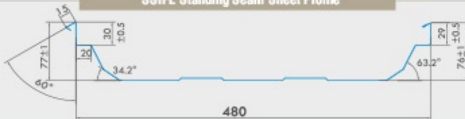
SSIPL Standing Seam Sheet Profile
