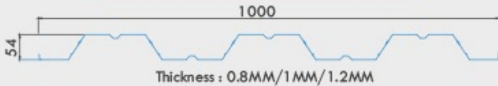
SSIPL Standing Seam Sheet Profile
